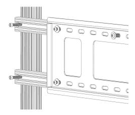
If vertical adjustment are necessary reposition the horizontal mounting extrusions with the fasteners in place and refasten to the vertical mounting extrusions. Level the wall bracket while retightening move to step 2F if horizontal adjustments are needed.
