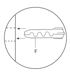
C Insert wall anchors (F) into hole.
