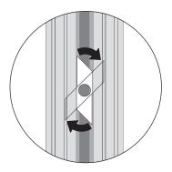
Insert Drop-In Nut (B) into the slots of the vertical mounting post and using the provided Hex Key.
