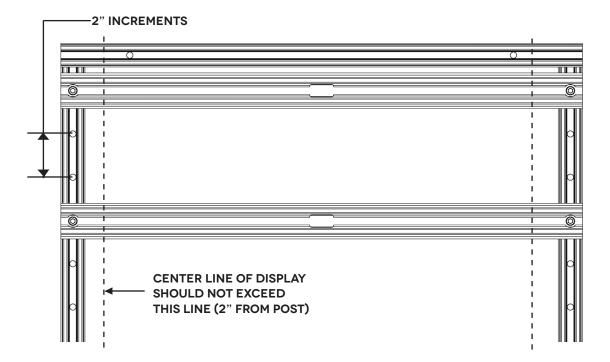
\*\* The Diagram above show the horizontal mounting extrusions without mount plates for visual clarification \*\*
