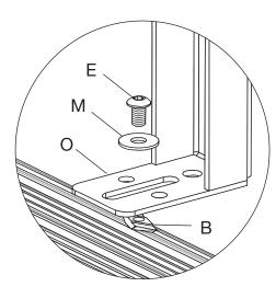
Loosely mount Bracket (O) using Screw (E), Washer (M) and Drop-In Nut (B).
