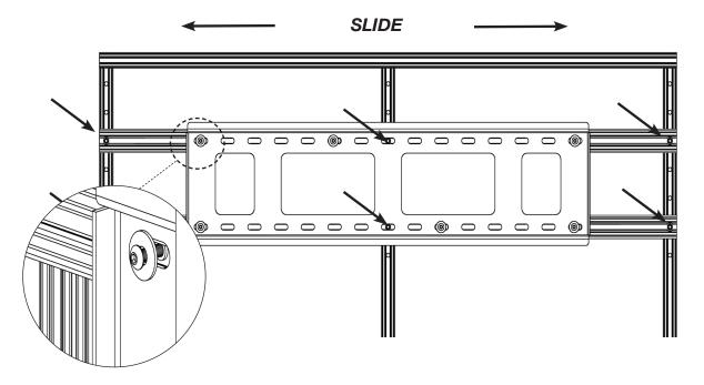
Loosen bolts fastening the horizontal mounting extrusions to vertical mounting extrusions. The flat nuts at the back of the vertical mounting extrusions will drop and need to be repositioned.
