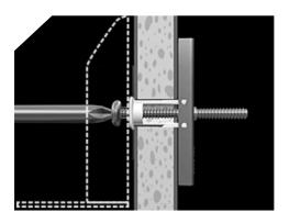
Move cabinet to wall and attach bracket. Insert bolt through Bracket and tighten until snug against wall.
