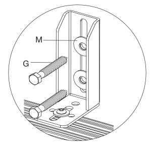
Place cabinet in place and fasten with washers (M) and Lag Bolts (G).
