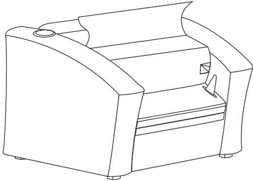
**A.** Lay backrest face down on seat and open lower access flap to expose mechanism receivers.
