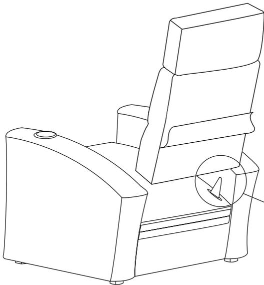
**B.** While holding access flap open, align mechanism backrest tongues protruding from seat with seat back receivers. Be careful to insert both sides simultaneously.
