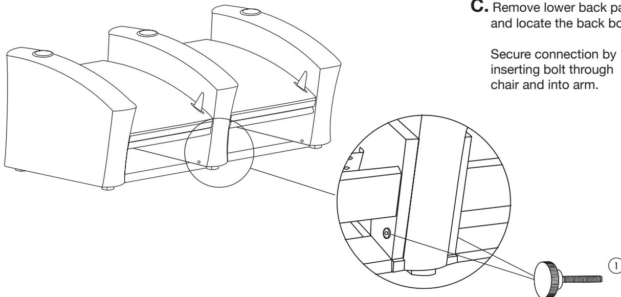
**C.** Remove lower back panel and locate the back bolt hole.
