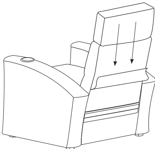
**C.** Press down evenly with both hands on backrest to be sure the clips in the backrest are engaged and fasten the backrest flap with the hook and loop fastener to complete the installation.
