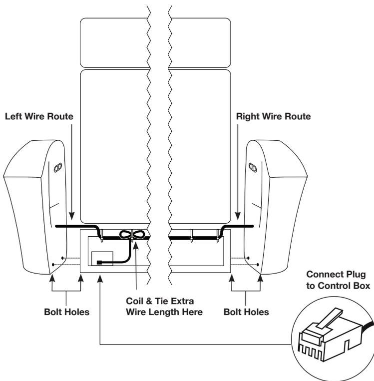
**A.** Align seats and connectors prior to assembly. Attention to switch location is necessary.
