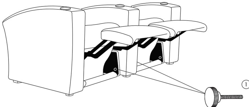
**B.** Extend foot rest to access front bolt holes and secure connection by inserting bolts through chair and into arm.
