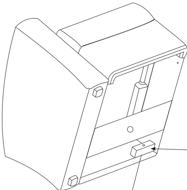
For powered seating connect power supply to jack located at the front of the control box under the chair.
