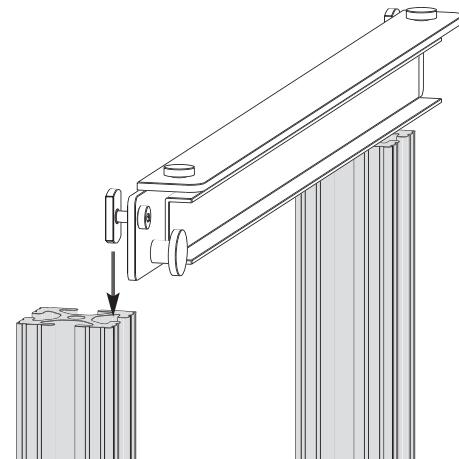
C. Insert the Rubber Tabs into the 2 holes on the shorter part of the bracket with the flat side facing up.
