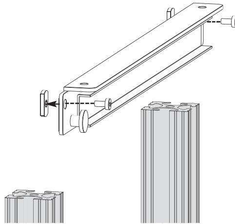
B. Insert the weld nuts into the channels making sure that the rollers face the front of the rack. Use the Spacer Tool provided and the instructions on opposite side to help space the drawer(s) as desired.
